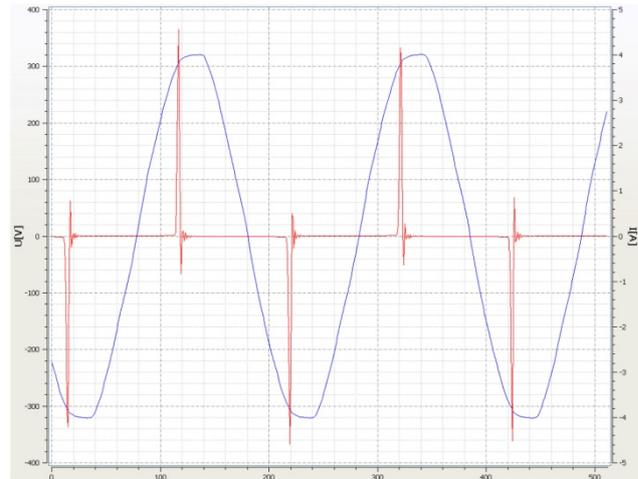
Many electronic consumers such as bridge rectifier circuits or switching power supplies have a high  $\cos \varphi$  that is close to 1, but a bad power factor.
