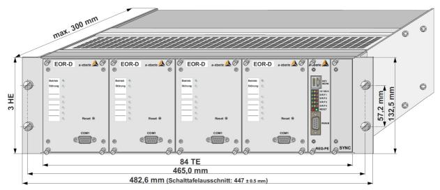
*Figure 12:* 84 TE rack containing four EOR-D for monitoring 16 control outputs including serial connection to the control (REG-PE)
