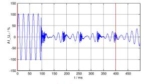
Figure 2: Voltage of the faulty conductor
