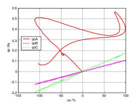
*Figure 1: qu-graph for a low impedance earth fault*
