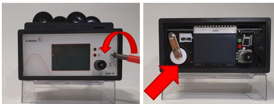
Figure 3: Removing the protection-paper between the contact and the battery
