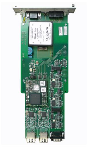
Picture 5: Electrical (RJ453) version of B1 release.
