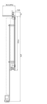
Picture 3: Dimensions plug-in module at B1 release
