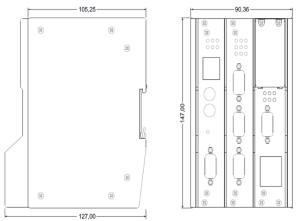
Picture 1: Dimensions rack at B3 release
