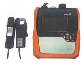
One sample with serial "1642-004" and firmware "MCU V3.009" was tested with a declared input voltage and current of  $U_{\rm din} = 230 \, \rm V$  and  $I_{\rm nom} = 20 \, \rm A$  and a nominal frequency of  $f_{\rm nom} = 50 \, \rm Hz$ .
