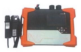
One sample with serial "1643-108" and firmware "MCU V3.009" was tested with a declared input voltage and current of  $U_{\rm din} = 230 \, \rm V$  and  $I_{\rm nom} = 20 \, \rm A$  and a nominal frequency of  $f_{\rm nom} = 50 \, \rm Hz$ .
