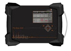
One sample of PQ-Box 200 with serial "1643-108" and firmware "MCU V3.009" was tested, the manufacturer states that this sample is representative of the PQ-Box 300 series. The device was tested with a declared input voltage and current of  $U_{\rm din} = 230$  V and  $I_{\rm nom} = 20$  A and a nominal frequency of  $f_{\rm nom} = 50$  Hz.
