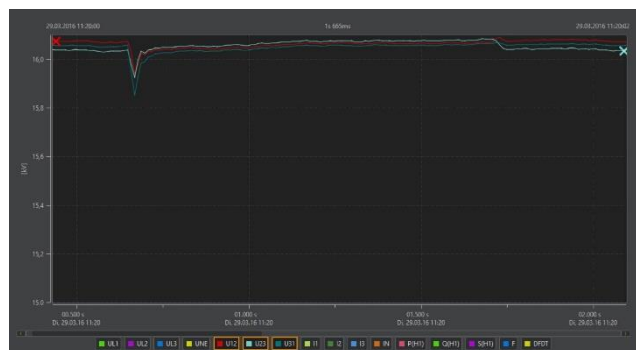
Figure 5 Recorder as 10 msec. RMS value U12, U23, U31
