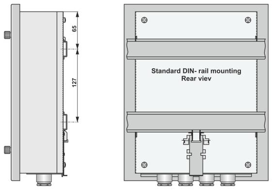
Figure 15: Mechanical dimensions, standard DIN-rail assembling
