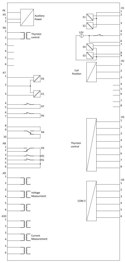
*Figure 26: Terminal connections CCI*
