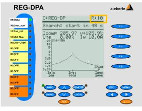
Figure 6: R:10 = Number of possible resistor cycles
