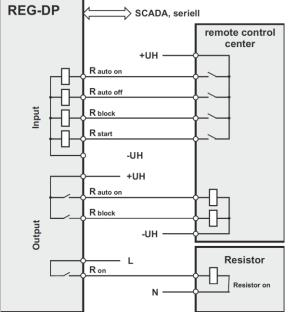
Figure 5: Example for the resistor control
