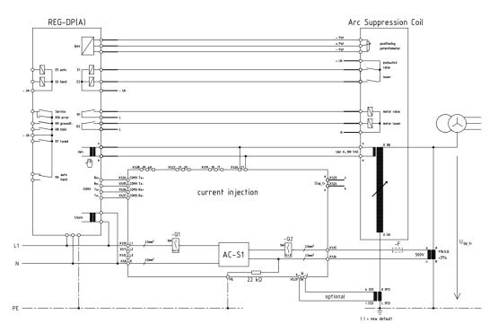
*Figure 23:* External power auxiliary winding and use of internal voltage transducer for the Petersen coil
