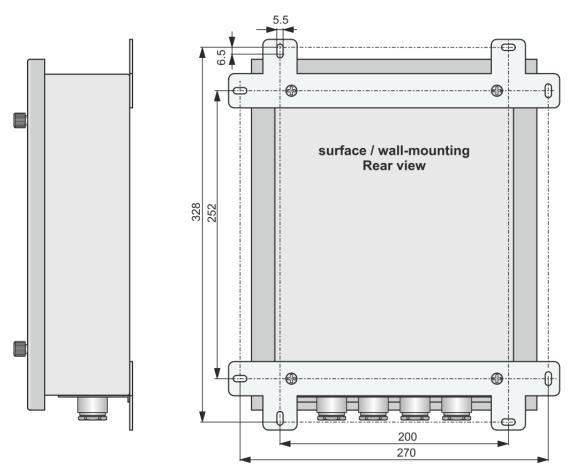
Figure 16: Mechanical dimensions, wall-mounting version
