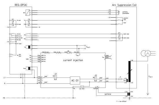
10.4.1 Connections to measure  $U_{\text{o}}$  at open delta winding
