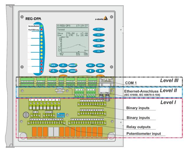
Figure 11: Location of the connector terminals
