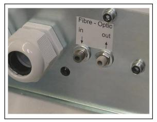
Figure 10: Fibre optic (FSMA-connection)
