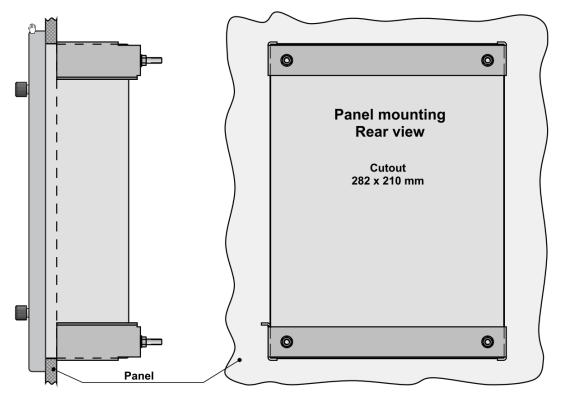
*Figure 14: Mechanical dimensions, Panel mount housing*
