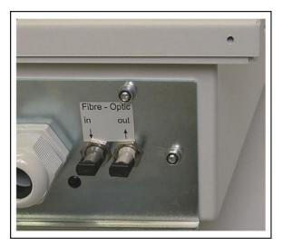
*Figure 9: Fiber optic (ST-connection)*
