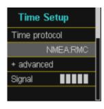
The signal quality is illustrated as a bar diagram in "Time Setup". At least one filled bar needs to be visible. In other cases, the synchronization precision lies at  $\pm$ 1 s.
