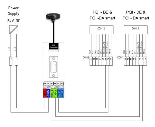
Establish the electrical connection between GPS converter and PQI:
