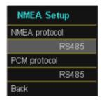
Set the NMEA and PCM protocol to "RS485" in "advanced" menu and return to "Time Setup".
