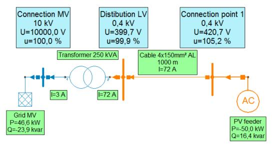
Figure 7-8 Low voltage grid with voltage boost along the cable (example)
