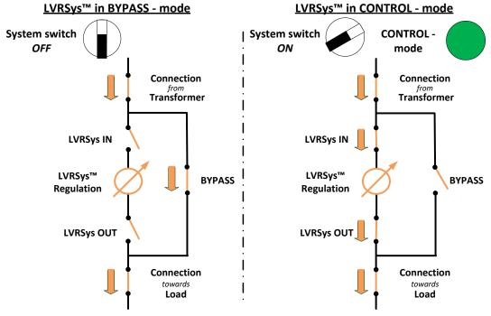
Figure 8-3 Circuit principle Bypass and operation
