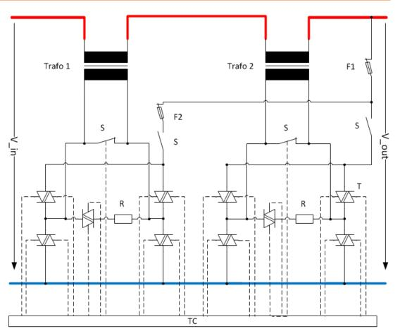
Figure 7-1 Single-phase functional diagram
