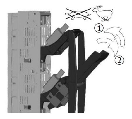
Figure 8-6 Operation switch disconnectors
