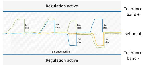
Figure 9-14 Example of unbalanced phase voltages
