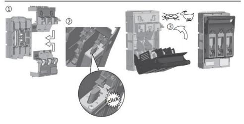
Figure 8-8 Operation fuse switch disconnectors
