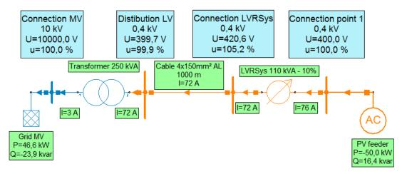
*Figure 7-9 Low voltage grid with voltage boost along the cable regulated through LVRSys* [Simulation Screenshots made with Neplan<sup>®</sup>].
