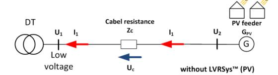
Figure 7-7 Low voltage grid with voltage boost along the cable
