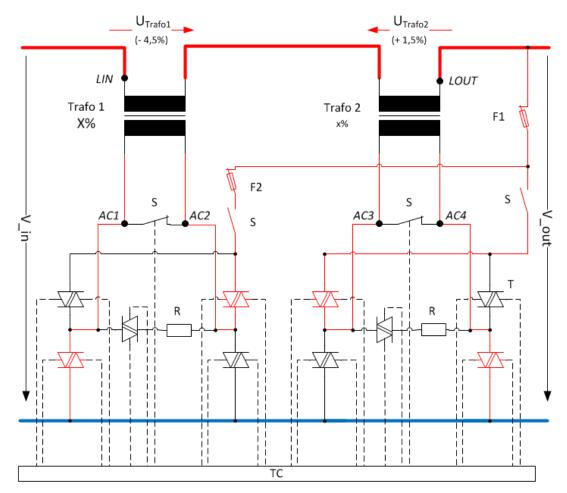
Figure 7-2 Example of 3% voltage reduction
