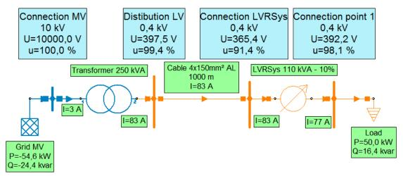
Figure 7-6 Low voltage grid with voltage drop along the cable regulated through LVRSys
