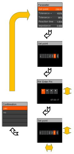
Figure 9-9 Setting the regulator parameters
