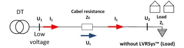
Figure 7-4 Low voltage grid with voltage drop along the cable
