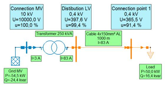
Figure 7-5 Low voltage grid with voltage drop along the cable (example)
