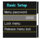
Access to the device setup can be disabled via a four digit password.
