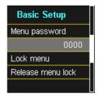
If a password is assigned, no access to the device set-up via the display is possible
