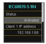
You can setup the device address and client address directly in the display menu.
