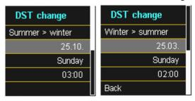
Menu for setting the parameters for daylight savings changes.
