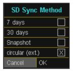
Confirm with "OK" and the PQI-DA *smart* will start automatically to copy the selected internal memory onto the SD card.
