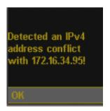
As of firmware version v2.6.0, the PQI-DA smart supports double IP address detection. Therefore, already assigned IP addresses of the subnet cannot be used. In this case, the wizard must be run again.
