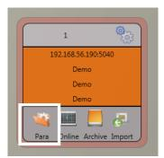
The PQI-DA *smart's* parameter setup can be accessed via **Para** button on the device panel. Parameters can be set in basic or expert view, which is also referred to as the classic view in the following sections. These views can be switched by choosing the corresponding selection field in the right main menu of the parameterization window.
