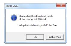
The REG-DA bootloader has its own interface parameters. These are visible after starting the bootloader. The baudrate can be set using the F3 key. The settings for flow control (handshake) and parity cannot be selected.
