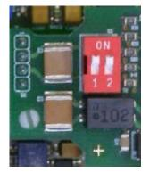
The three-wire or four-wire circuit is selected through two DIP switches on the resistor input module (feature E97/98) or next to terminal 23 (feature D2/3/5/6/8).
