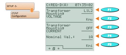
In this menu one can determine which phase-to-phase and current will be used for measurement.
