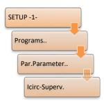
In addition to the tap difference, the master-follower parallel program monitors circulating reactive current via lcirc-Supervision. If the lcirc limit is exceeded, the parallel error ParErr is generated. (also see Chapter 8.2.7.7 Parallel operation error (ParErr), page 234)
