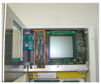
Installed analog module
