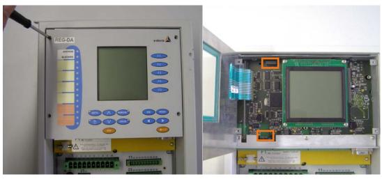
Loosen the front panel of the REG-DA
