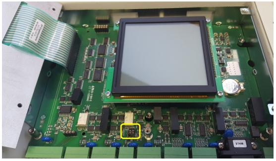
REG-DA with open front panel, DCF jumper position marked
