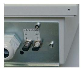
Fibre optical connection (ST-connector, V17, V19)
