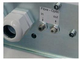
Fibre optical connection (FSMA-connector, V13, V15)
