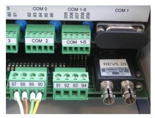
Fibre optical connection (1 x Ethernet-ST, XW93) at Level II; REG-DA Com ports at Level III
