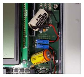
Parallel plugged batteries; hold down bracket removed
