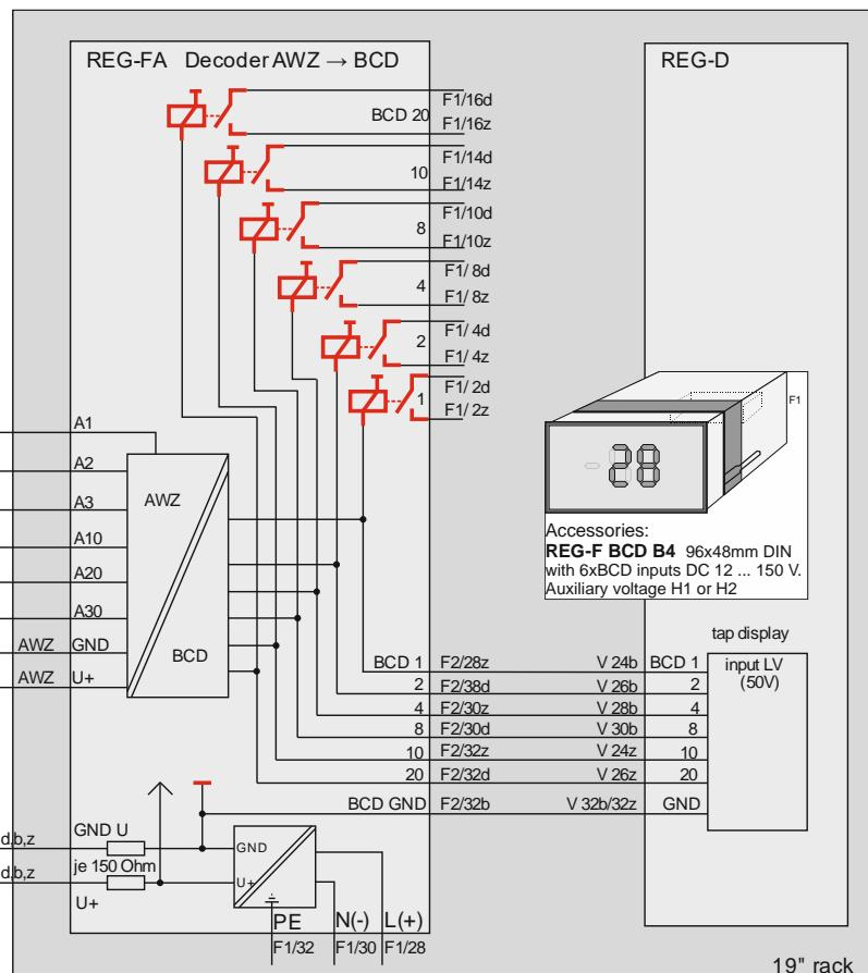
For longer distances between REG-FA and the tap changer row, the maximum cable length is less due to the DC resistance (see example), but rather determined by interference from parallel cables. A superimposed AC voltage up to 2V at the REG-FA input is allowed. Each application has different earthing and voltage conditions. The only general statement that can be made, with shielded cables and greater distance to the parallel cables, a longer distance is possible.
