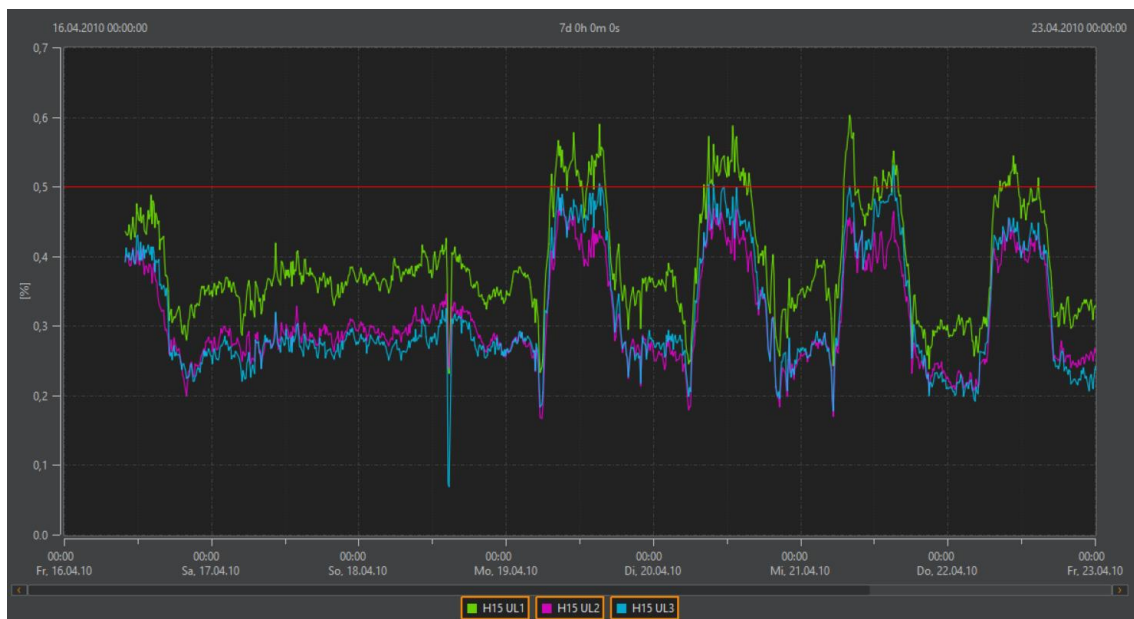
Figure 3: Voltage curve and entered limit values in WinPQ mobile
