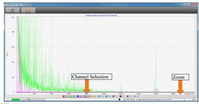
Using the zoom function it is possible to adjust the scaling of the application.
