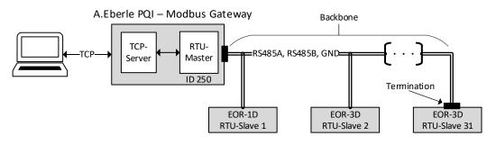
Figure 1: Exemplary connection of a RS485 bus with Modbus gateway
