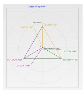
In the vector diagram, connection faults are easy to detect. All phase voltages and currents are displayed with phase angles.
