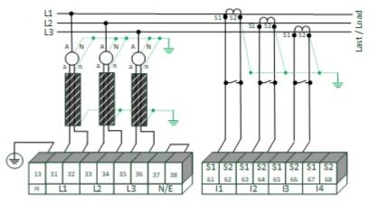
PQI-DE in three-wire connection for medium and high-voltage networks via voltage sensors
