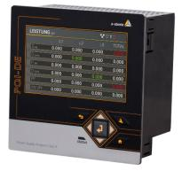
Pressing the "right" and "left" keys on the keypad will change the side of the numeric display.
