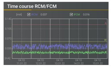
Diagram of the residual current (RCM) and fault current (FCM) over the last 7 days Selectable curves:
