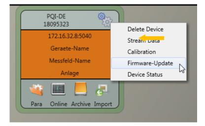
The **General setup** device function tile can be used to carry out a firmware update for the PQI-DE measuring device.
