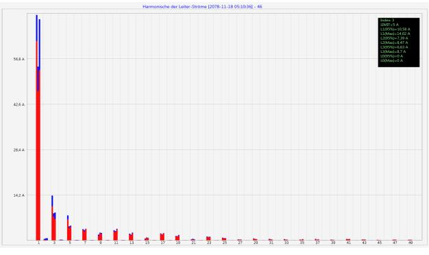
Example: Statistic current harmonics 2nd to 50th - scaling in ampere
