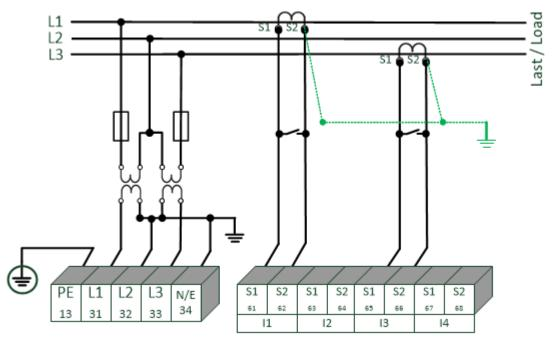
*PQI-DE* in the V-circuit / Aron circuit for medium and high voltage networks via converters with L2 grounded
