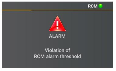
If the set alarm threshold is exceeded (see chapter 6.5.2), a visual alarm message must appear on the display according to DIN EN 62020.
