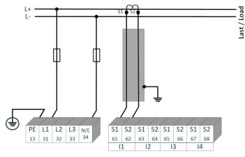
Example connection PQI-DEt with current transformer with small signal output (e.g. 4V)
