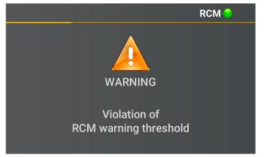
If the set warning threshold is exceeded (see chapter 6.5.2), a visual alarm message must appear on the display according to DIN EN 62020.
