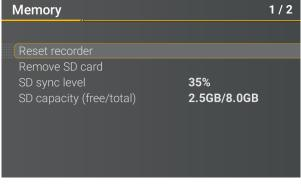
**T**o remove the memory card, operate the "Remove SD card "function.
