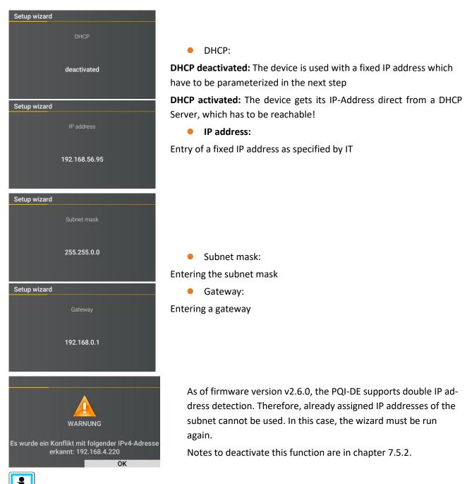
In the factory setting, the PQI-DE is factory pre-set with the IP address 192.168.56.95 and the subnet mask 255.255.0.0.
