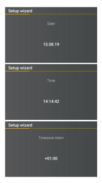
Manual entry of date and time as local time. Furthermore the local time zone must be entered and if the device should calculate the changeover for summer / winter time by its own
