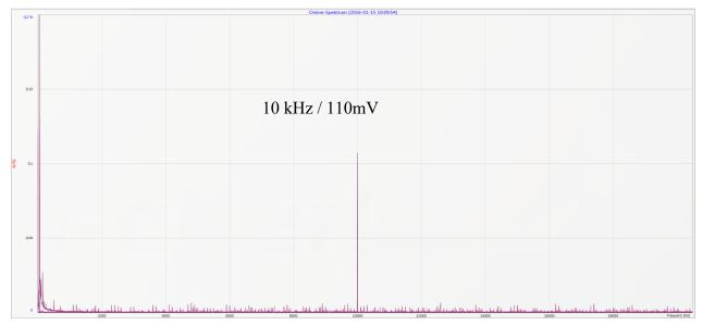
Example: charging device for electrical cars / 10 kHz sampling frequency visible in the FFT analysis.
