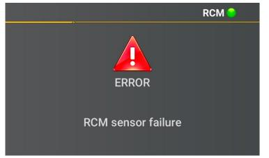
If an error occurs (e.g. wire breakage in the differential current transformer) an error message is displayed.
