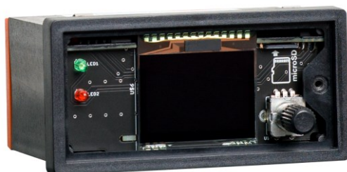
Figure 6: EOR-1DS with demounted front plate for SD card access
