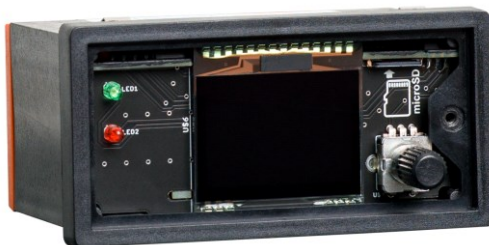
Figure 4: EOR-1DS with demounted front plate for SD card access
