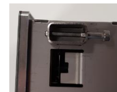
Mounting bracket engaged on PQI-DE
