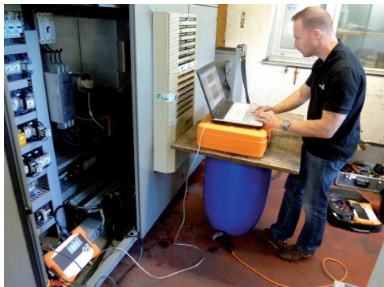
Figure 6: PQ-Box 200 mains analyser set up on the CNC machine.
