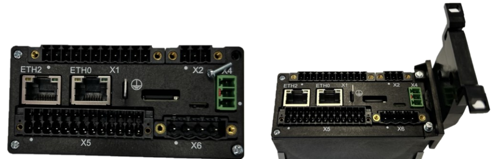
Montage Hutschieneadapter an das EOR-3DS
