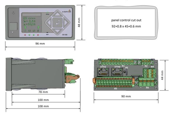
Figure 15: Dimensions EOR-3DS with feature U05/U06/U07 with C10
