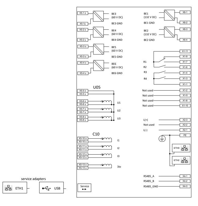
Figure 20: EOR-3DS terminal assignment for feature combination C10 and U05
