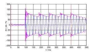
Figure 3:  $u_0(t)$  with a restriking fault
