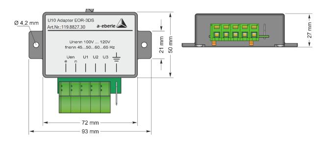
Figure 18: Dimensions of voltage measurement adapter for 100 V / 110 V transducers; order code U10
