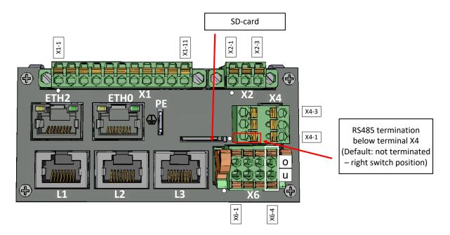
Figure 13: Voltage and current measurement inputs via RJ45, SD-card and RS485 termination switch with features C29/U29 or C31/U31
