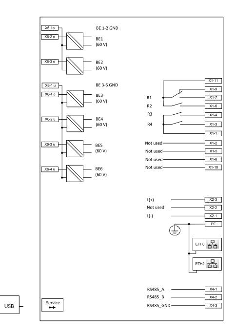
Figure 28: EOR-3DS terminal assignment for feature combination COO and UOO
