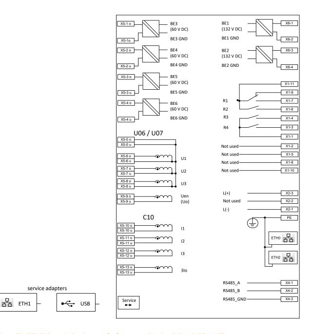
Figure 22: EOR-3DS terminal assignment for feature combination C10 and U06 or U07
