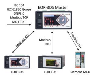
For switch gears, where a motor control unit (MCU) is installed for switching of circuit breakers, this way it is possible to connect MCU units via Modbus.
