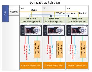
Figure 4: Cross calibration for one feeder
