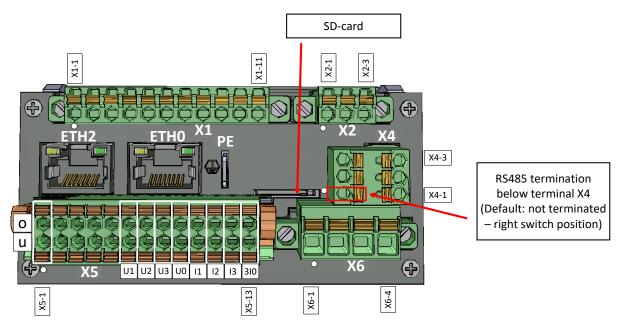
Figure 12: Terminal location for voltage and current inputs, SD-card and RS485 termination switch with features U05/U06/U07/U10 with C10/C21/C25
