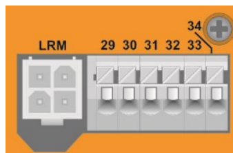
LRM interface on the back of the EOR-1DS
